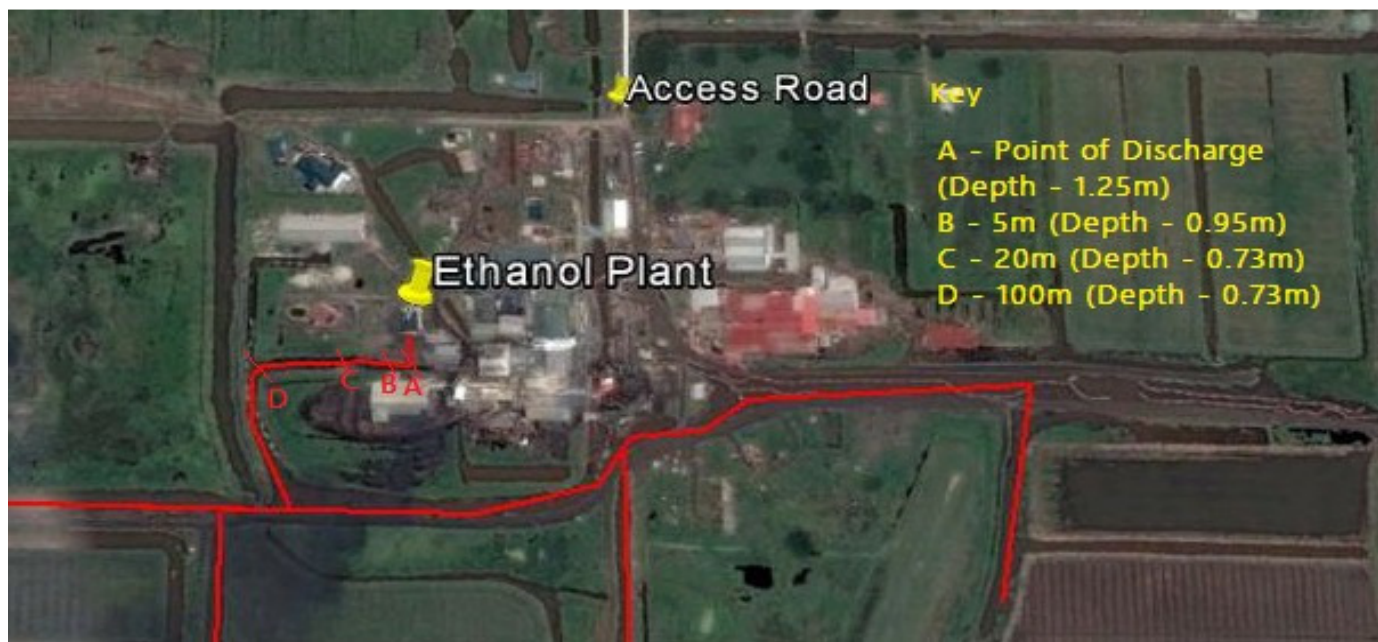
Figure 1: Layout of the Albion Bioethanol Plant with the Sampling Points and Varying Depth Readings (Source: Google Earth, 2013)
