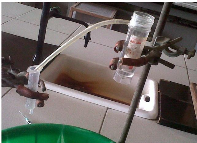
Plate 1: Locally Constructed Analog Plethysmograph
