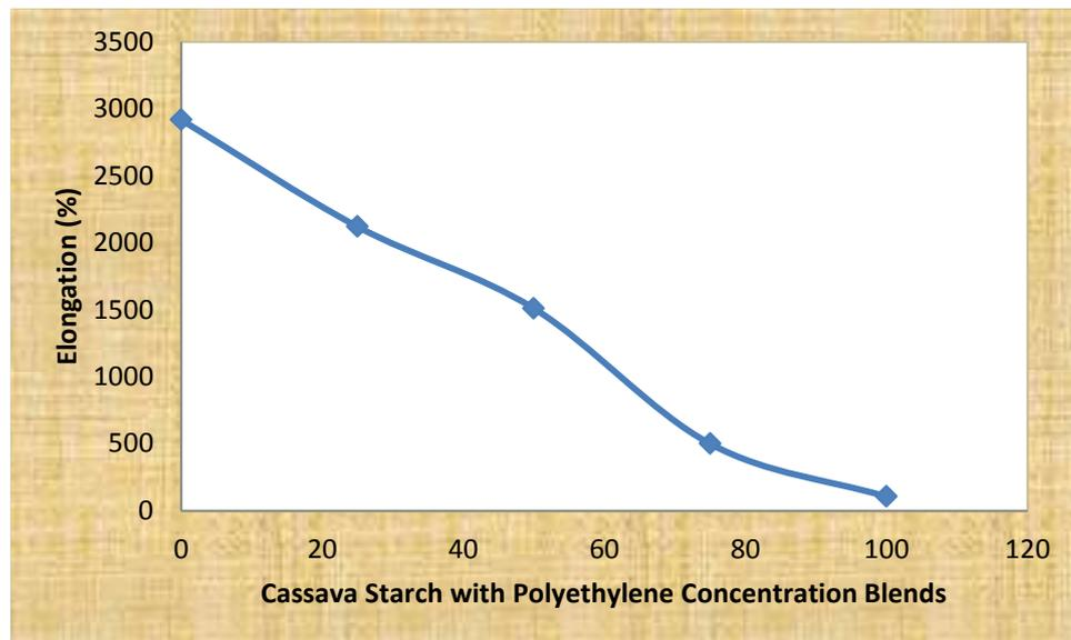
Figure 5: Elongation percentage of Biodegradable Polymer Blend with Polyethylene
