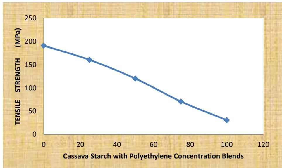
Figure 6: Tensile Strength Responses of Biodegradable Polymer Blend with Polyethylene
