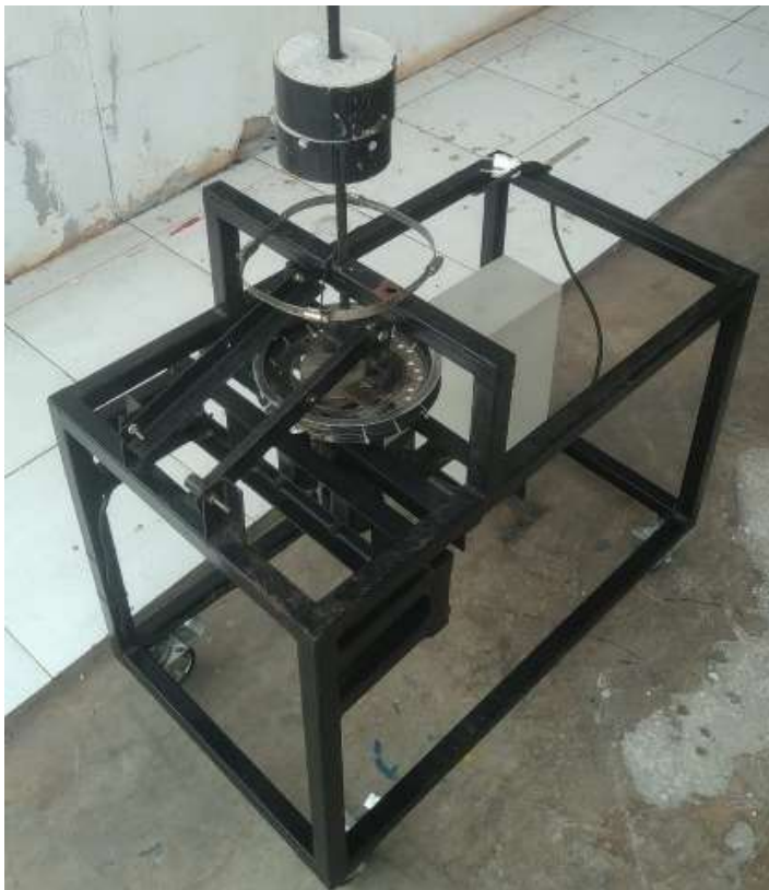
Figure 4. wear test equipment and wear test direction
