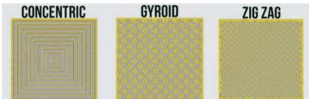
Figure 2. Geometric infill shape.
