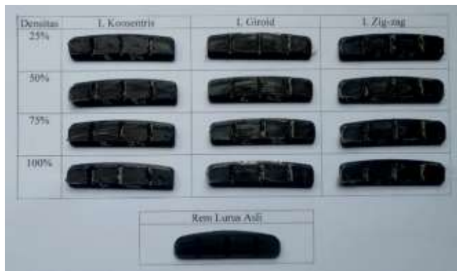
Figure 8. TPU brakes after wear testing
