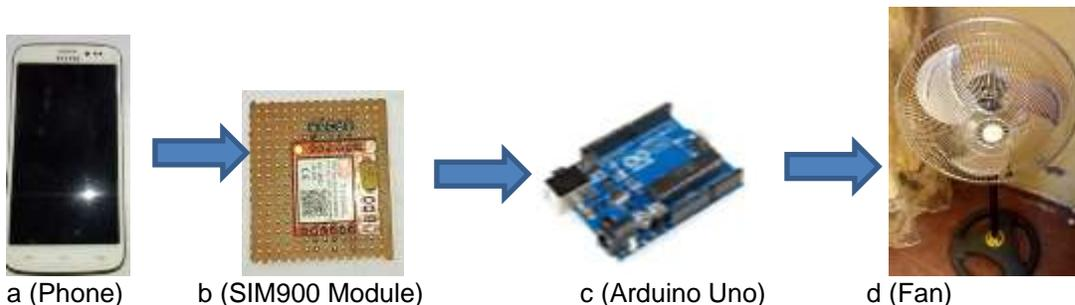
**Figure 1. Proposed diagram of the SMS Home Automation System**
