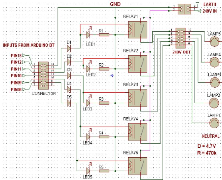
Figure 4. 5V -240 V switching circuit of the relay board [6]
