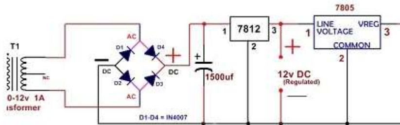
Figure 5. Circuit diagram of the Power supply unit.
