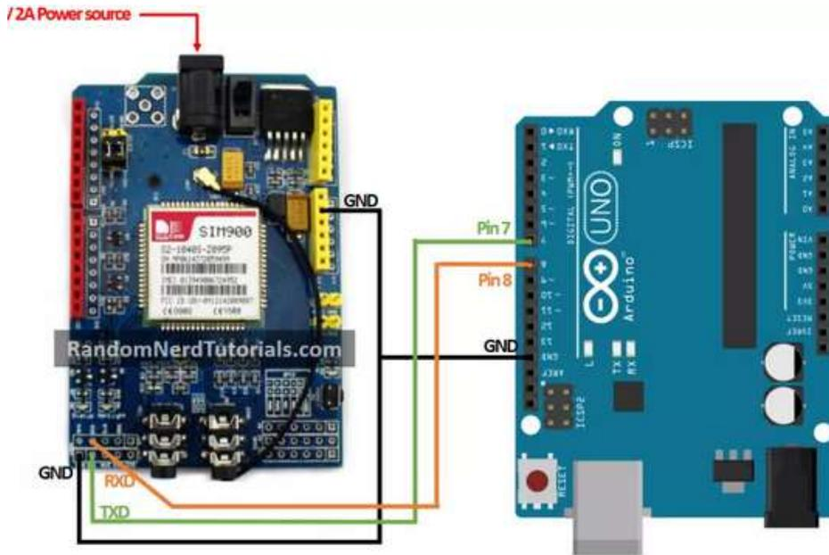
Figure 2. Interfacing GSM SIM 900 Module with Arduino [ 3].
