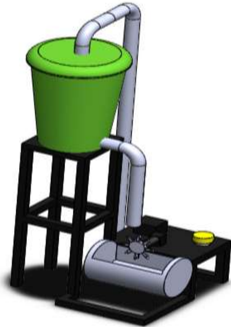
Figure 3.5: The Mini Hydro Power Plant
